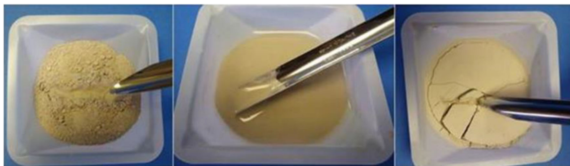
Fig. 1 Qualitative caking test using untreated rock dust. Left: dry rock dust; center: water mixed with rock dust; right: rock dust after water evaporates
