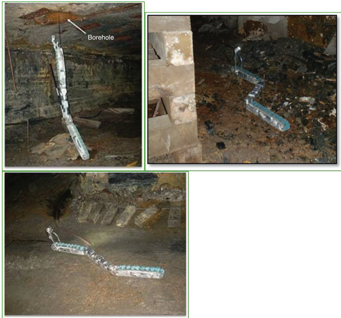
FIGURE 4 Snake robot lowered through borehole, then traversing a mine floor with coal and rock debris.
