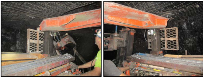
Figure 4. Locations of MSHA-requested respirable dust sampling. The left/return operator sampler corresponds with the wet box collector (left). The right/intake operator sampler corresponds with the dry box collector (right).
