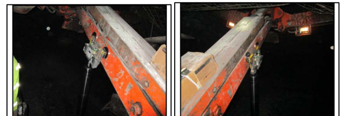
Figure 3. Location of the gravimetric samplers for the left/return side bolter (left) and the right/intake side bolter (right).
