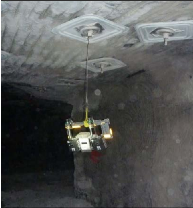
Figure 5. A typical gravimetric sampling package consisting of a pDR-1000 and two gravimetric samplers. This package is typically hung from a roof bolt or mounted on mining equipment.
