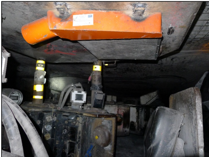
Figure 1. Air curtain plenum welded to underside of ramcar canopy located above the operator's seat.
