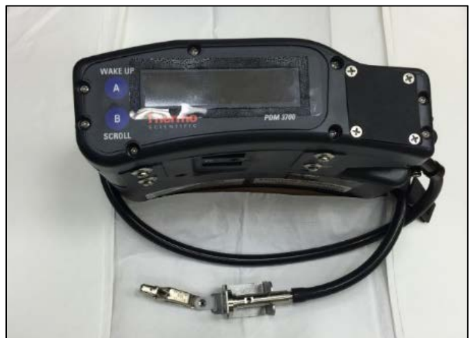
Figure 4. A PDM 3700 respirable dust sampler.
