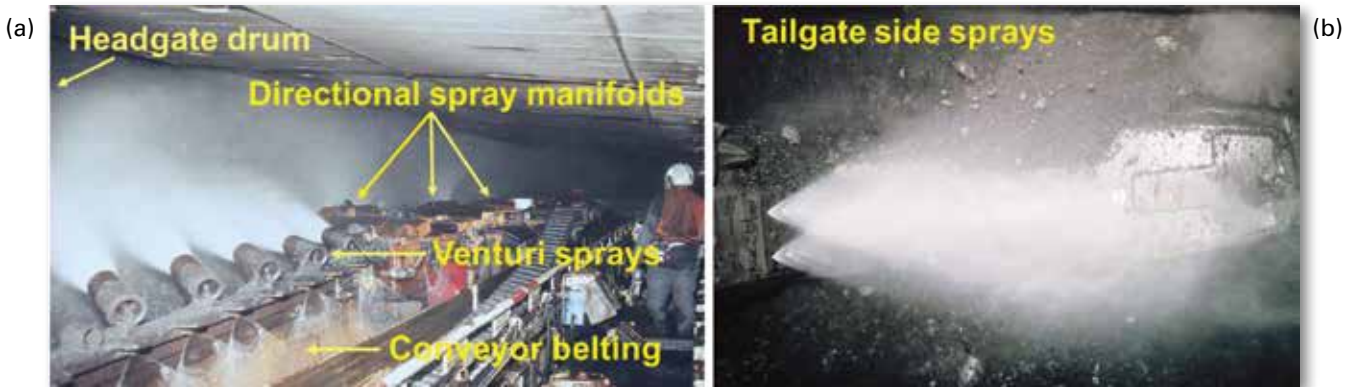
Fig. 2 (a) Directional spray system on longwall shearer with venturi sprays mounted on the splitter arm and hollow-cone sprays on shearer body, and (b) tailgate-side sprays.
