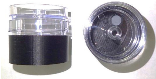
Fig. 4 The picture on the left shows a side view and the one on the right shows the top view of the high-sensitivity cassette
