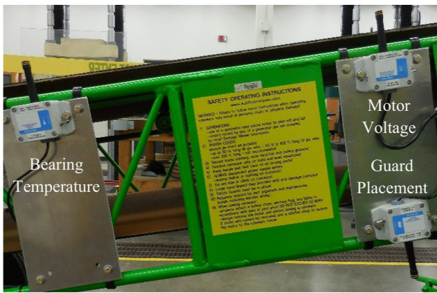
Fig. 6 Sensor nodes installed on a conveyor
