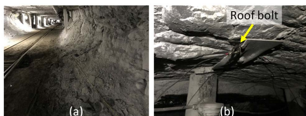
Fig. 2 TTE measurements in an underground coal mine. (a) shows a picture of the mine entry in the underground, and (b) shows one of the roof bolts used as the electrode for TTE signaling.
