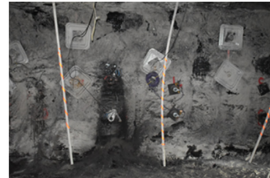
Fig. 5. Instrumentation type and location for the cross-cut side of instrumented pillar at site-1.
