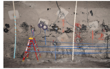
Fig. 4. Instrumentation type and location for the entry side of the instrumented pillar at site-1.
