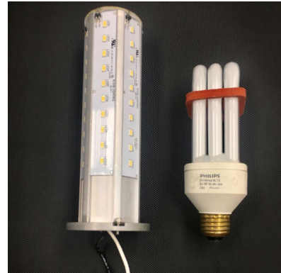
Figure 2. The replacement LED lamp (left) and the legacy CFL lamp (right).
