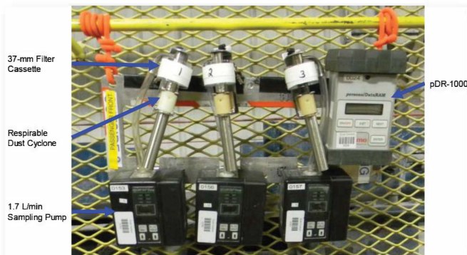
Fig. 2 Example of sampling racks with one pDR-1000 and three gravimetric sampling assemblies, including sampling pump, respirable dust cyclone and 37-mm filter cassette.
