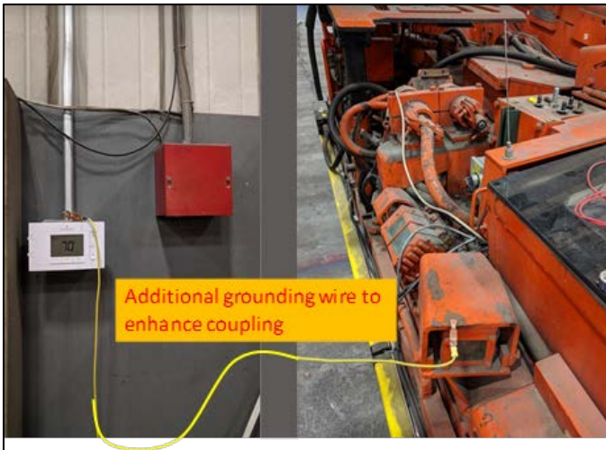
Figure 3. The metal frame of the CMM is connected to a metallic pipe on the wall of the building to enhance the parasitic coupling.
