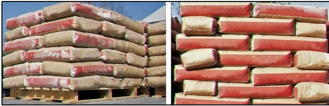
Figure 8. Pallet of bags without being cleaned by the B&BCD system (left) and with being cleaned by the system (right).
