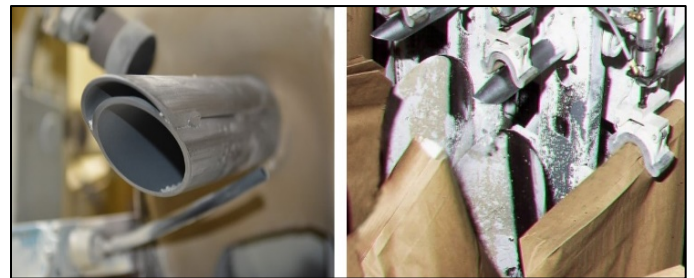
Figure 6. Photos of dual-nozzle system (left) and improved bag clamp design (right).
