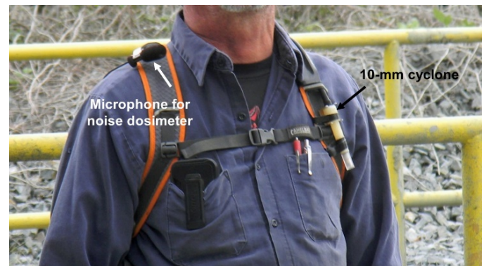
Figure 3. Simultaneous assessment of a miner's respirable dust and noise exposure using the Helmet-CAM system.
