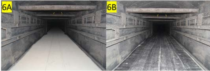
Figure 6A. Rock dust distributed on the floor; 6B: Rock dust topped with coal dust before the explosion.
