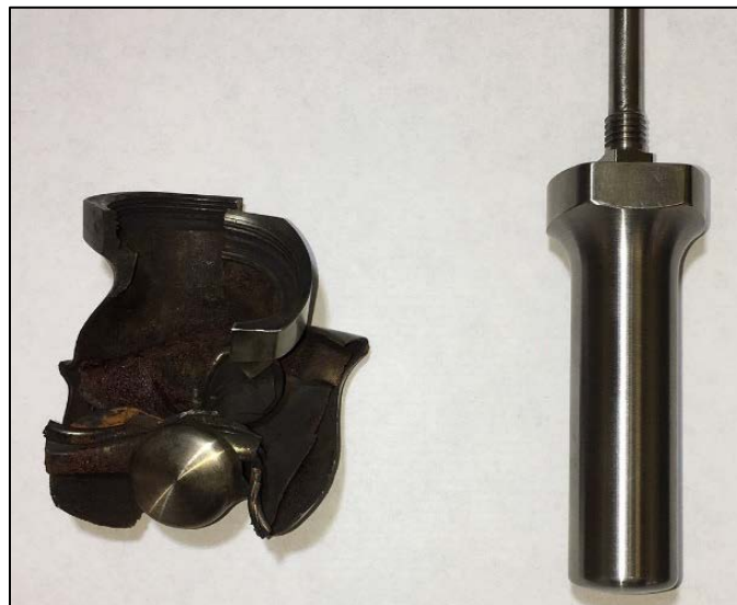
Figure 5. The ruptured 19.6-mL canister next to an undamaged canister.
