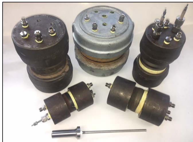
Figure 1. Canisters provided varying amounts of free space around enclosed Li-ion cells.
