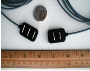
Fig. 2. Single and double differential electrodes
