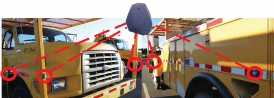
Fig. 7. Sensor deployment locations for the truck.
