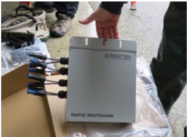
Fig. 16 Rapid shutdown device for a residential project
