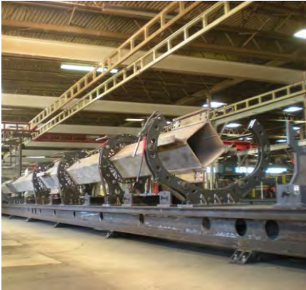
ConXTech fabrication shop with rotating clamps www.prweb.com/releases/conxtech/ladbs-approved/prweb10762433.htm
