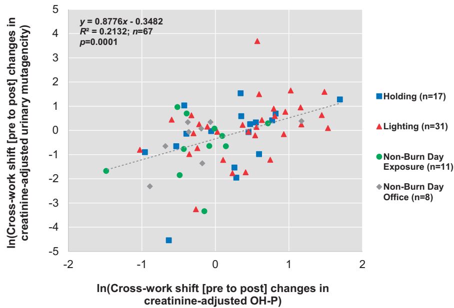
Figure 6. Correlation between log-transformed cross-work shift (pre- to post-) changes in creatinine-adjusted urinary mutagenicity and log-transformed creatinine-adjusted OH-pyrene. Person days are indicated as n . Linear mixed effect model results showed a positive significant correlation ( p = 0.0001 ).
