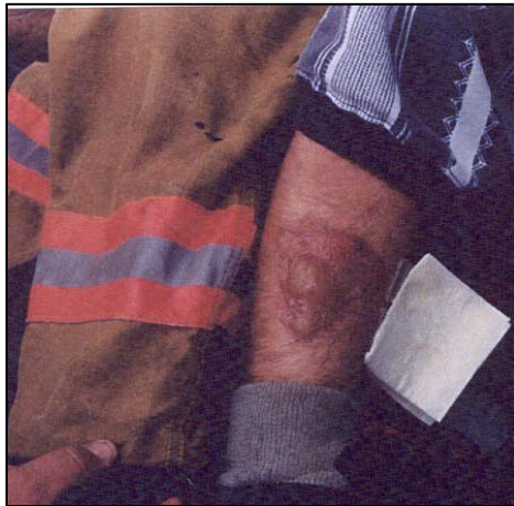
Figure 3. Burn Injury observed behind reflective trim attached to sleeve of a turnout coat and reported in reference [2]
