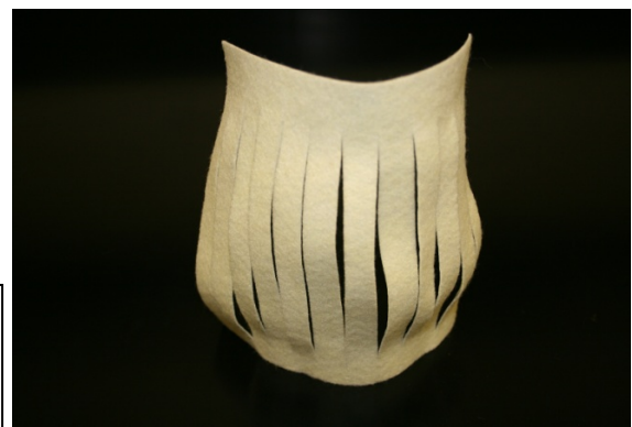
Figure 16. Moisture barrier sample with cuts to increase moisture vapor permeability
