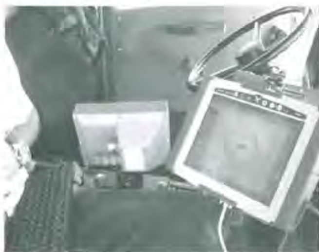
Figure 2 — Photograph showing the installed rugged flat panel computer in a CAT 793 truck.
