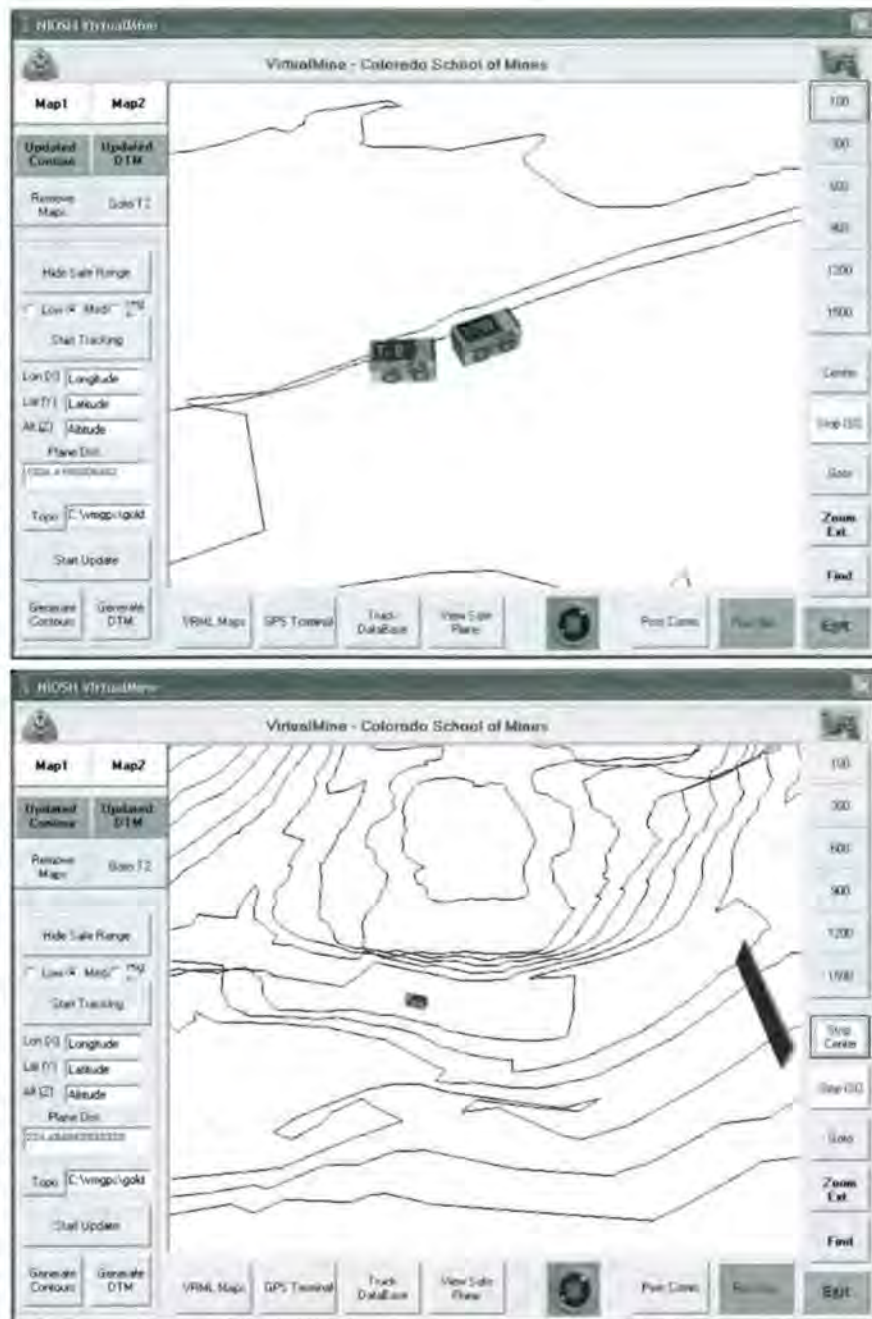
Figure 8 — Three-dimensional isometric views showing the position of trucks being monitored by VirtualMine on a given contour map.
