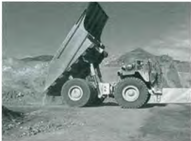
Figure 18 — The mine truck during the dumping process based on the new updated map that was radio transmitted from the dozer.
