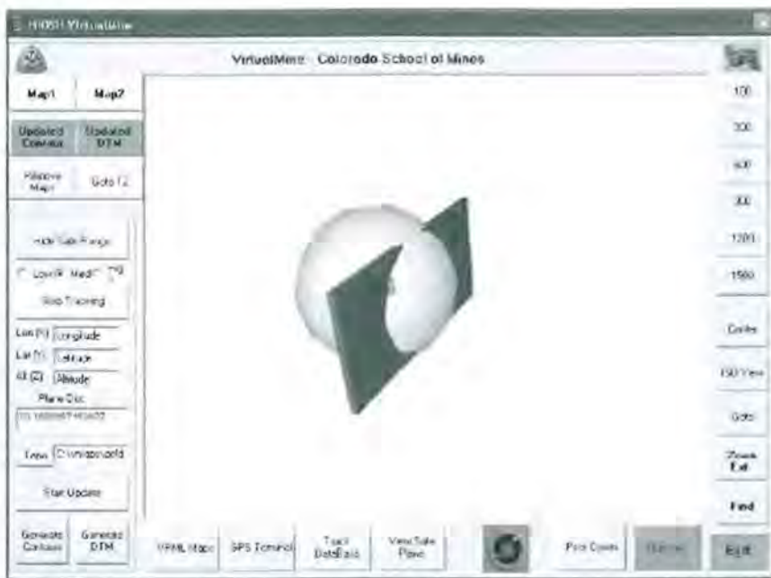
Figure 9 — Three-dimensional safety sphere (truck inside) intersecting with the safety virtual berm (plane).
