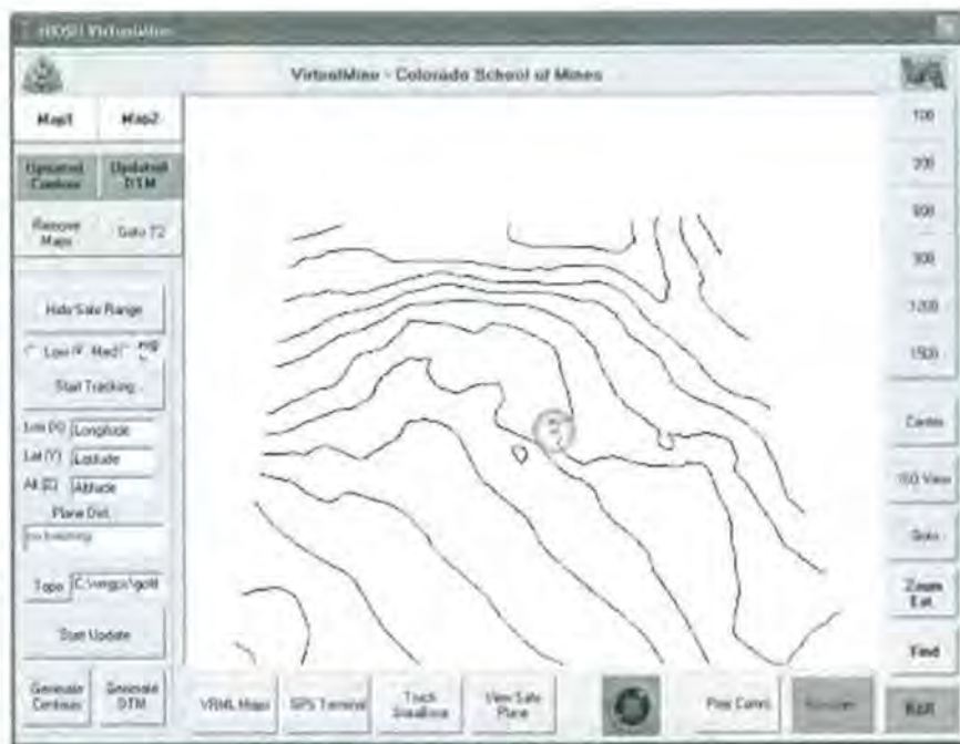
Figure 11 — Three-dimensional contour map generated on-demand by driving at the CSM campus.
