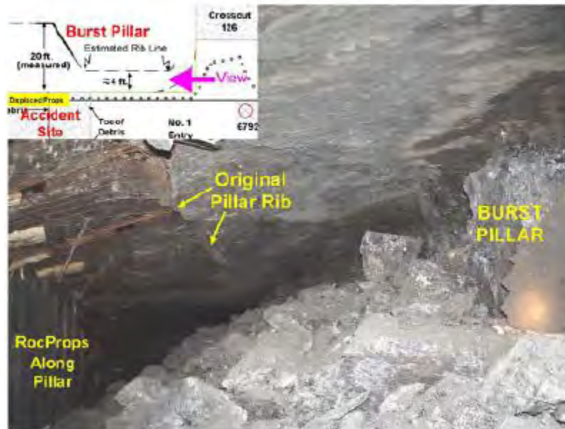
Figure 2.3: Example of a crush-type unstable failure of a Crandall Canyon coal pillar after massive bump event. Void space can be seen where coal was ejected from the original pillar [116].
