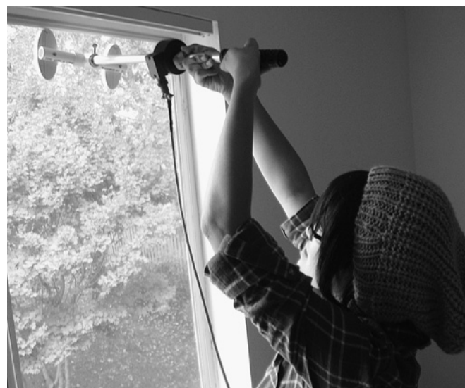
Figure 1 Testing screen failure threshold with static load.
