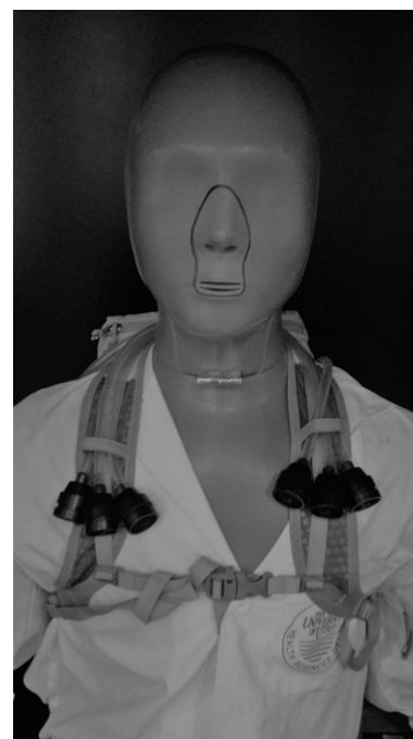
Figure 3. New samplers ( n = 6 ) draped over the manikin shoulders at approximately 45° angle downward from the horizontal.
