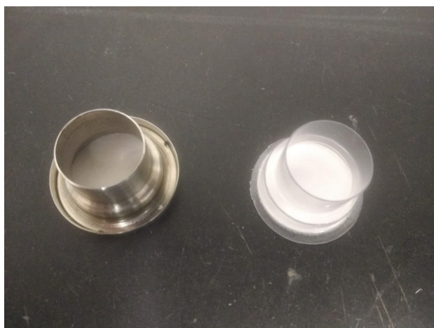
Figure 2. Side-by-side comparison of the IOM cassette (left) and the capsule-style filter of the new sampler (right).
