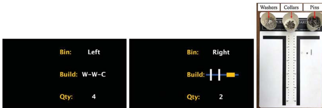
Fig. 2. Illustration of text-based (Left) and graphic-based (Middle) information, and the simulated assembly task involving a Purdue Pegboard (Right). In the information displays, “Bin” indicates the column of the pegboard in which washers, collars, and pins are assembled, while “Build” indicates the sequence of washers (W) and collars (C) on a pin.
