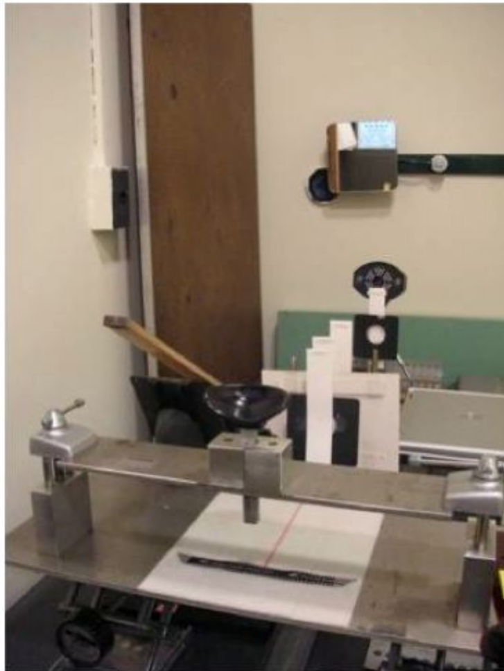
Figure 5. Outcome Measure Workstation Setup. Plusoptix Power Refractor II (the black oval-shaped device close to the wall) was placed 1 meter away from the subject's eye (about where the black chin rest was). The distant target was presented in the mirror with an equivalent viewing distance of 4 meters. The slanted wood ruler was placed to the left and in front of the chin rest for a more accurate NPC measurement.
