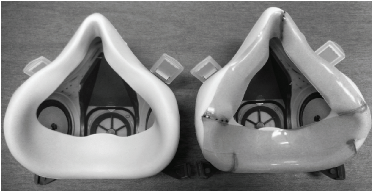
Figure 5- 2. A conventional elastomeric half-mask versus a modified elastomeric half-mask (same model).
