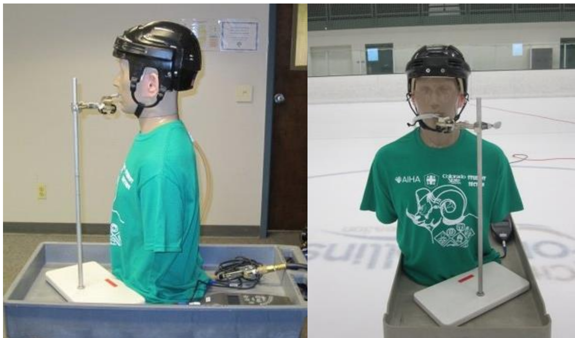
Figure 5.5: KEMAR sampling assembly (left) a. side view of KEMAR Type 45 BA assembly fitted with a Bauer hockey helmet, Fox 40 ® Super Force ® finger grip pea whistle apparatus, and the Larson Davis SLM/OBA; (right) b. front view of KEMAR assembly located on the ice at a northern Colorado ice rink
