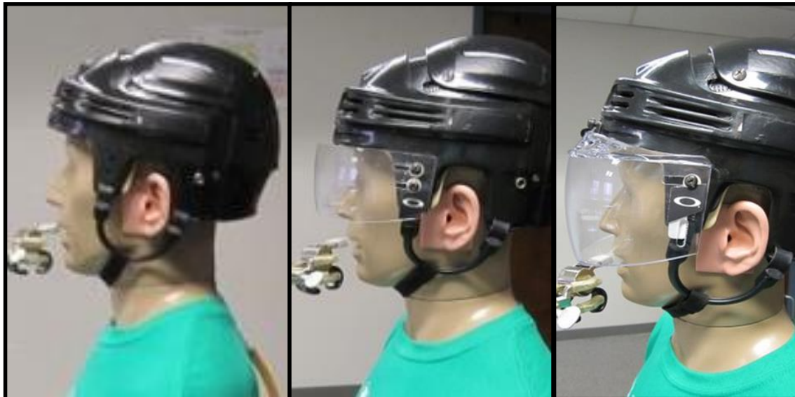
Figure 5.6: Hockey helmet configurations (left to right): a. Bauer ® 4500 hockey helmet without a visor; b. Bauer ® 4500 hockey helmet with a 2.75” Oakley ® VR904 modified straight small visor with slots; c. Bauer ® 4500 hockey helmet with a 4.0” Oakley ® VR924 CLE pro straight visor with vents
