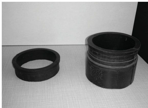
Figure 6.2: (Left) PVC flexible rubber coupler was cut to be 1.0 in. tall for the top of the dome (Right) PVC flexible rubber coupler was cut to be 3.0 in. tall for the bottom of the dome
