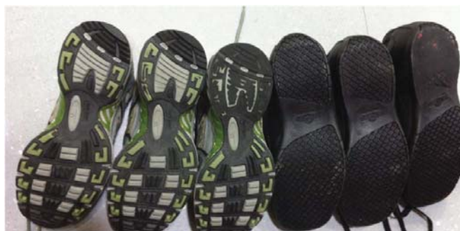
FIGURE 3 Shoes tested in this study from left to right: full-tread athletic, half-tread athletic, no-tread athletic, full-tread work, half-tread work, and no-tread work. Tread was only removed from the heel of the shoe as that was the contact region during slipping.
