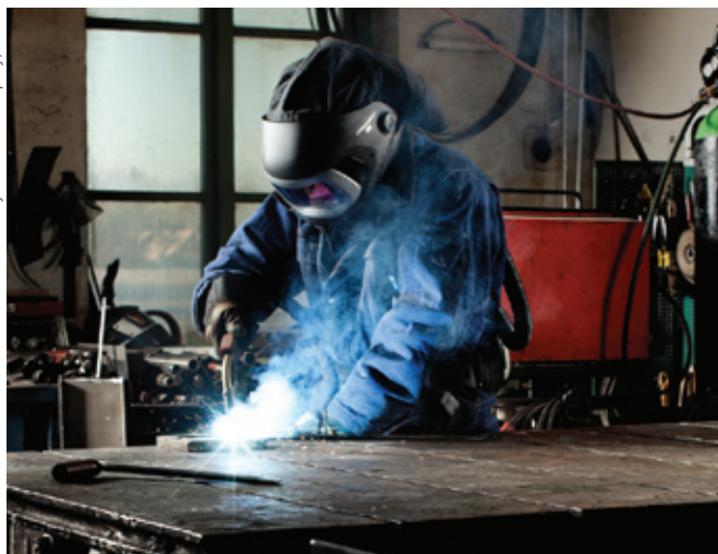
This 3M 9100 FX Air helmet protects workers from hazardous welding fumes with a built-in respirator (PAPR). Its auto-darkening visor can reduce neck strain from flipping visors down.
