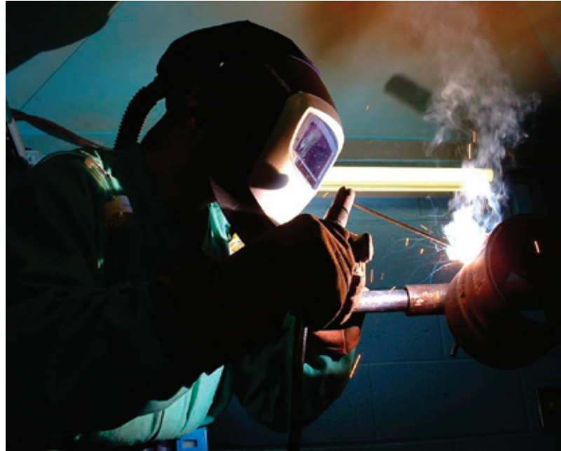
This welding hood with an integrated, battery-powered air-purifying respirator protects the welder from hazardous fumes.
