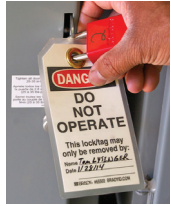
A machine being locked and tagged out
