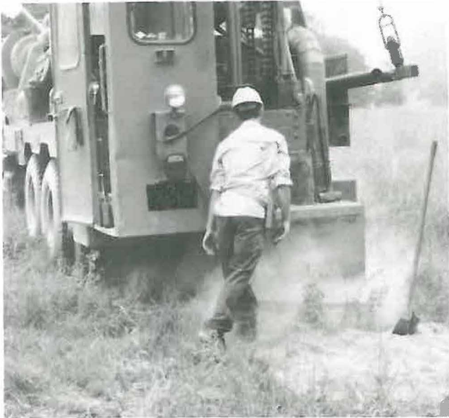
Figure 1. Rock driller working without respiratory protection on a mobile rig.
