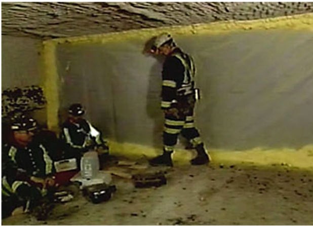
Fig. 1 A brattice cloth barricade with a foam sealing agent at the boundaries [11]
