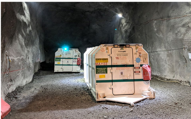
Fig. 3 Steel-structured safe haven [29]
