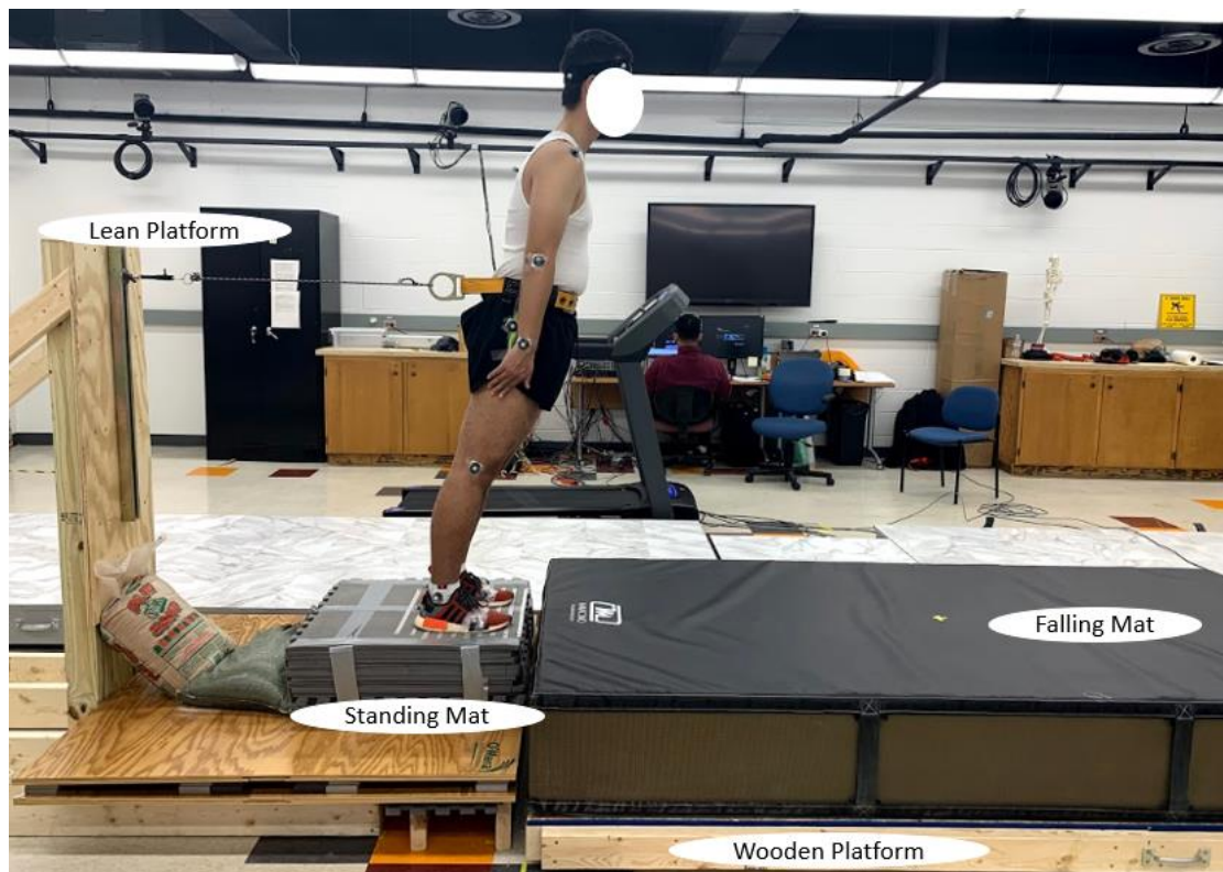
Figure 1. Setup used for forward falls from standing, with initial angle of 15^\circ . Setup for backward falls from standing was similar; the lean angle was set to 10^\circ , and participants were facing the opposite direction instead.
