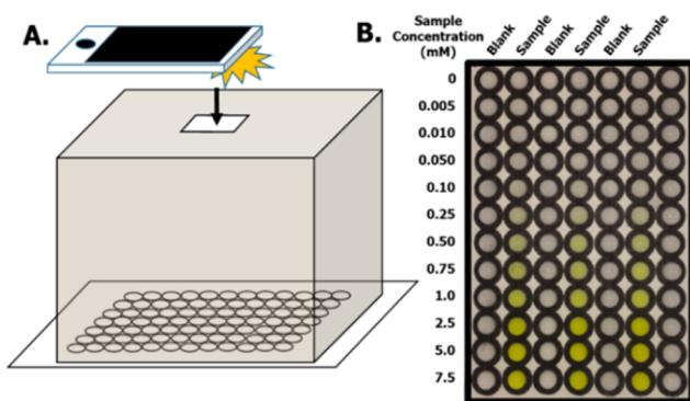
**Figure 3.** Scheme showing (A) the image capture process using a cellphone for the “light box” plate reading method and resulting (B) PNP calibration image labeled with blank and sample regions.
