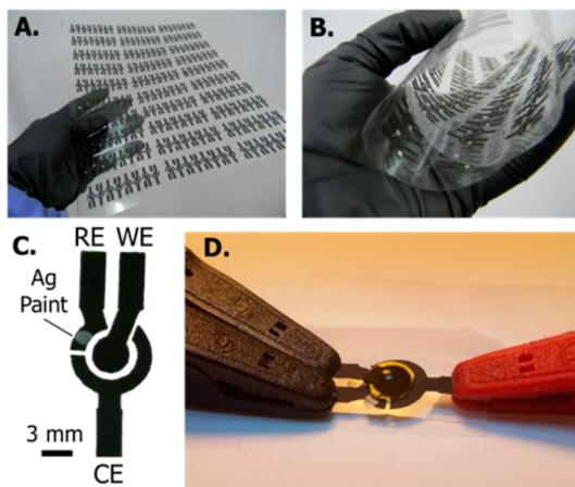
**Figure 2.** SPCEs on transparency film shown as (A) printed sheet that is (B) flexible. (C) A single printed electrode image (with background removed for visualization) showing working (WE), silver paint reference (RE), and counter (CE) electrode geometries and connections. (D) Final device image with 30  $\mu$ L of solution contained within the central well and connected to potentiostat leads.
