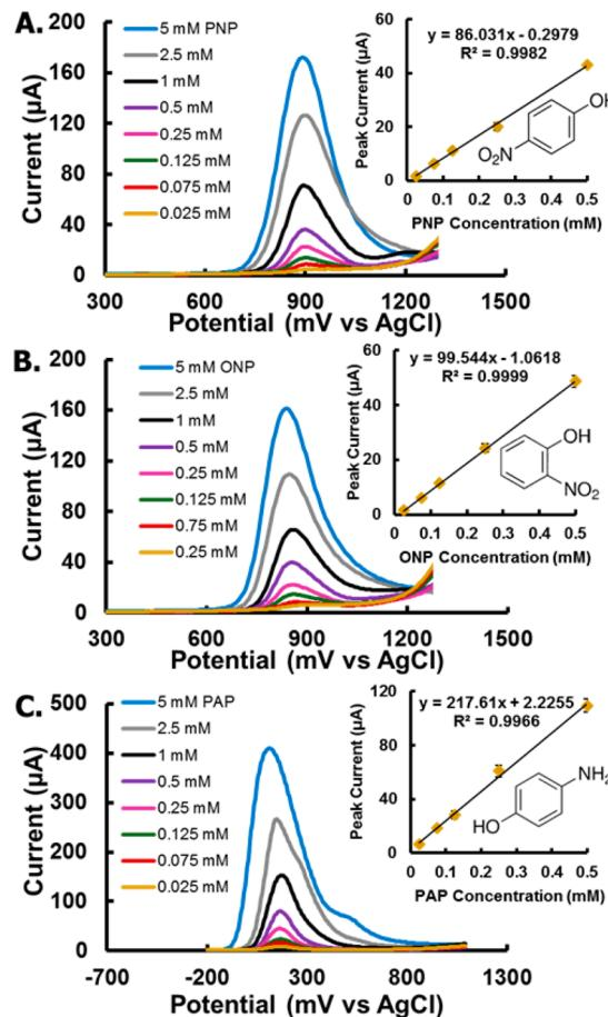
**Figure 4.** Optimal SWV settings used to measure and plot increasing concentrations of (A) PNP, (B) ONP, and (C) PAP detection along with the resulting linear range calibration plots in pH 6.5 PBS buffer ( $n = 3$ ).
