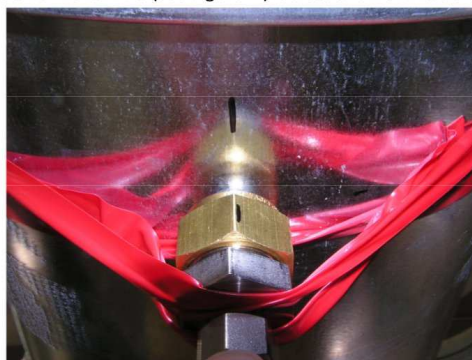
Use markings to ensure proper alignment
