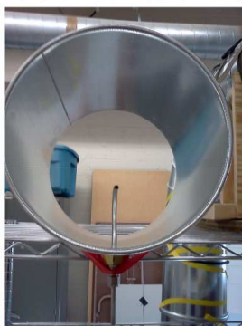
Internal view of isokinetic nozzle in a duct (duct is assembled this is just an illustration)
