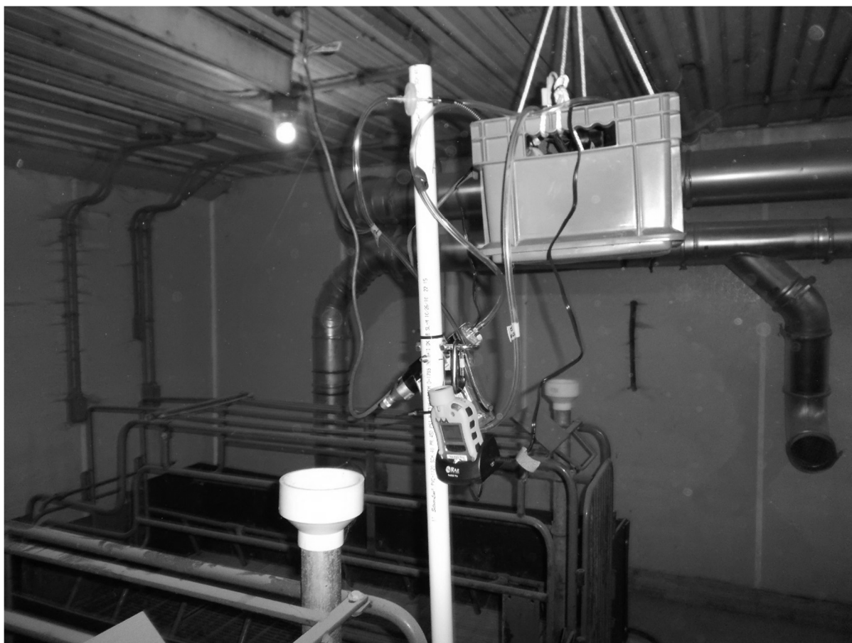
Figure 3: Direct-reading instrument deployment at Position A. Inlets of instruments were positioned 1.5 m from the floor. The ToxiRAE was attached to the pole. The VRAE was hung in a basket and the instrument tubing was fed through a bolt fastened to the pole.
