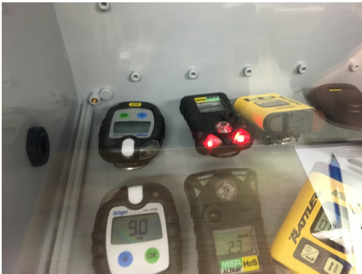
Figure C2. Upon initial charging of chamber during Run 7 (on equivalent barn day 64), the chamber was filled to a concentration of 10.5 ppm H 2 S, according to the ToxiRae inside. In response, the secondary Altair went into low alarm mode, but the primary Altair did not respond. This was the first alarm discrepancy observed between the two monitors.
