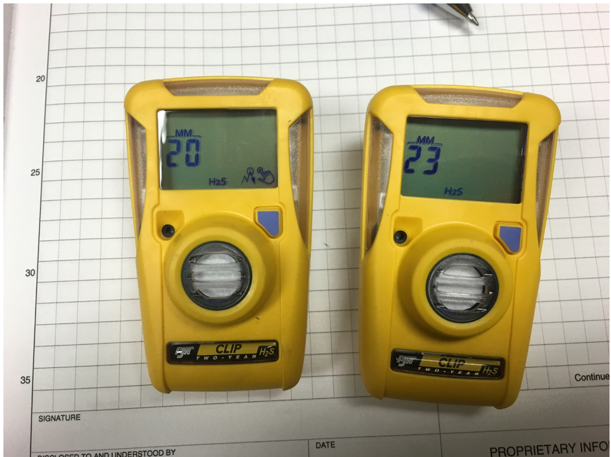
Figure C3. Activated simultaneously, the BW Clip on the left was the primary and on the right was the secondary monitor, which was stored within the hibernation chamber during the study. This photo shows the difference in countdown of 'months remaining' on the monitors' displays. The hibernation case had extended the life of the secondary by 3 months at this point in the study.
