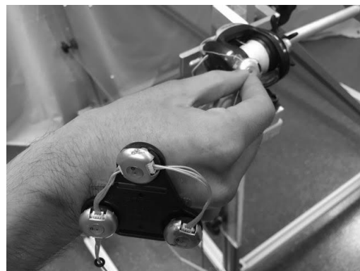
Figure 3: Pretest calibration to predict end effector position using the hand marker triad.
