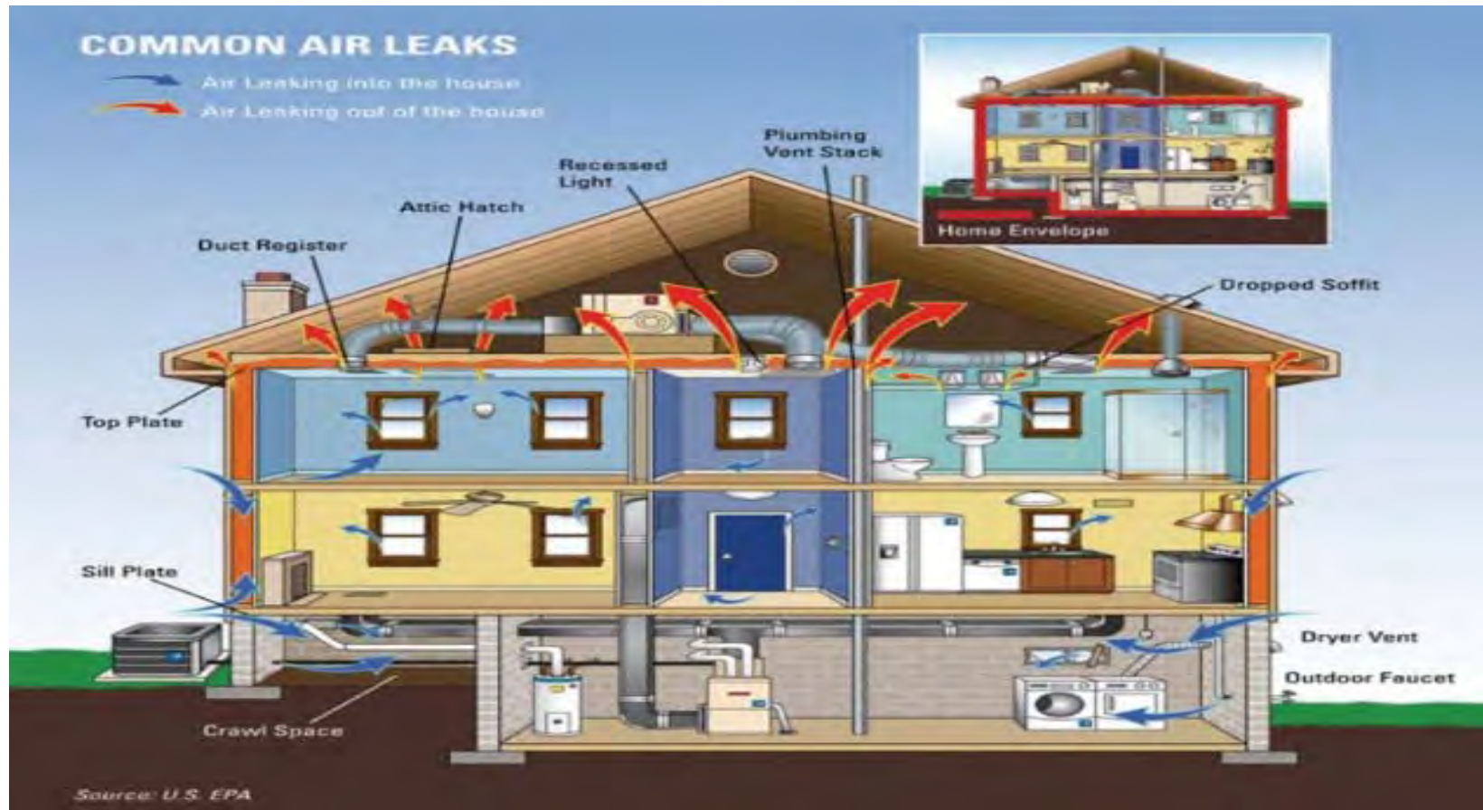
Common Air Leaks in a Building
