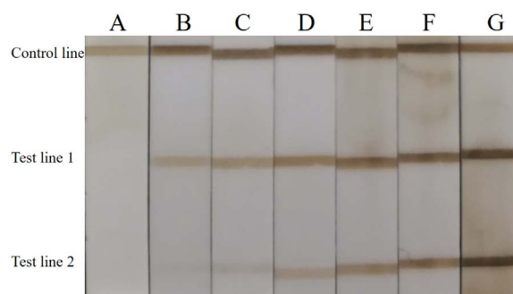
Fig. 4. Photographs of visual readout of the proposed ICA for the detections of carbaryl (test line 1) and chlorpyrifos (test line 2) both at (A) 100, (B) 50, (C) 20, (D) 10, (E) 5.0, (F) 0.1 and (G) 0 ng/mL.
