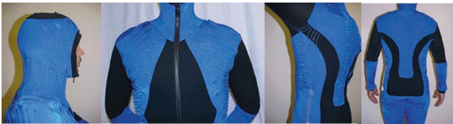
Fig. 7.1 Liquid cooling garment. (NPPTL/NIOSH photo archive)
