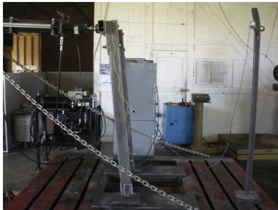
Fig. 2 – Rear load test Long 460 ROPS.
