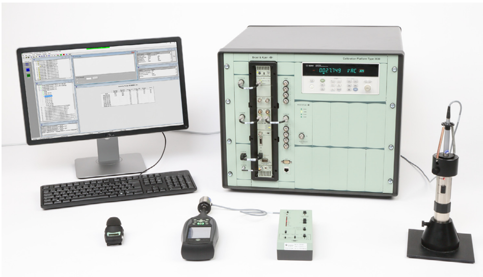
Fig. 1. Sound level meter calibration system Brüel & Kjær Type 3630.
