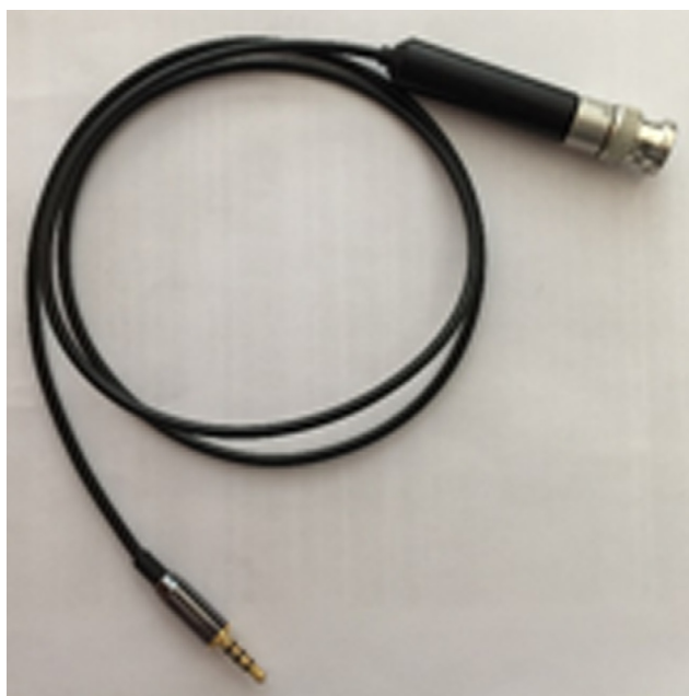
Fig. 3. Electrical substitution of external microphone.
