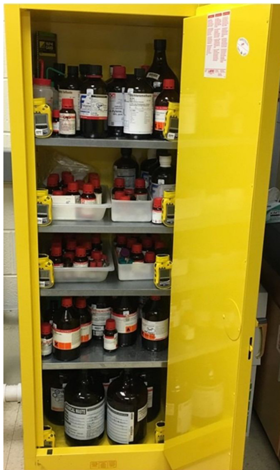
Figure 3. An array of PID gas sensors positioned along the front edges of 4 of 5 shelves of the LS316 FSC.
