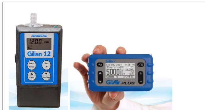
The Gilian 12 (20.5 oz) will pull 10 Lpm of air through the prototype sampler, and the GilAir plus (20.5 oz) will pull 2 Lpm through the IOM.
