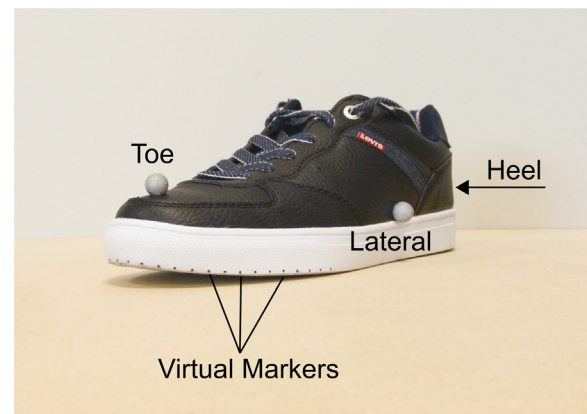
Fig. 2. Photograph of the shoes worn by subjects showing the placement of physical markers and virtual markers. The positions of the virtual markers were defined within a shoe-fixed coordinate system based upon the three physical markers shown.
